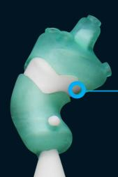
Effortless break-up of the cast form due to defined brittleness and easy peel-off when using the cast separator, especially for more complicated structures.
